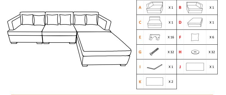
Attach the feet (E) to the bottom of each base piece (A, B, C & D). The feet are located in a zippered pocket on the underside of each base piece. Use 2 bolts (G) and washers (H) per foot using the pre-drilled holes.
